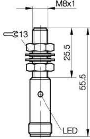
**Inductive Sensors** BES 516-343-E5-C-S 4 M8x1 x 55.5 normally-open **Sn=1,5mm** shielded
